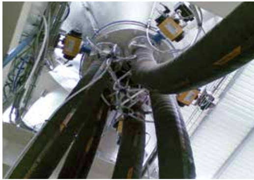
Micro-silica conveying 1 silo feeds 5 separate lines.
